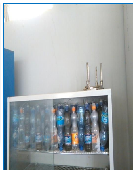
Figure 4. Digesters in the oven at 38°C
