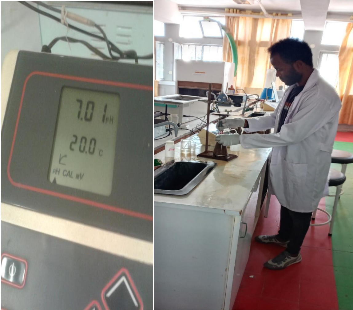
Figure 3 Arrangement of the pH measurement before anaerobic digestion of the substrates.
