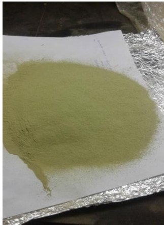
Figure 8. Drying the sample using an oven dryer, milling it, and sieving it were indicated .
