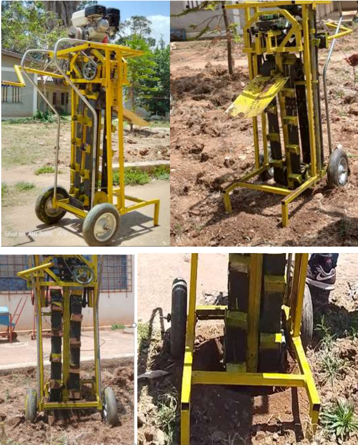
Appendix Figure2. Prototype of the motorized hole digger during testing
